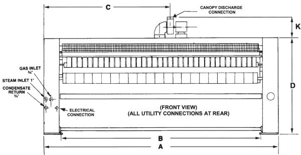
Allow minimum of 18" (457 mm) clearance at ends of machine for maintenance access. Canopy blower requires 10" diameter venting; 1050 CFM. Provide adequate make-up air according to current local requirements. Canopy vent must be independently discharged to atmosphere. Do not interconnect with other vent lines. Do not use for construction purposes unless certified correct by CMV Sharper Finish, Inc.
