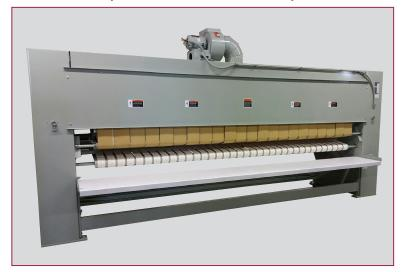
Convenient discharge height. Ironed work delivered to the rear of the machine is raised to a height of over 31" inches (787 mm) by discharge conveyor. This increased height allows this machine to be used with all automatic folding machines. In addition, if work is to be hand folded the increased height increases productivity and reduces operator fatigue. For increased height, 6" (152 mm) 'Frame Feet' are available.
