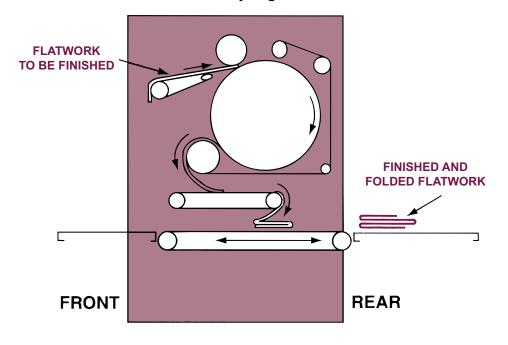
IRONED LINEN DE-LIVERD TO THE REAR AL-LOWS YOUR LAUNDRY TO MORE THAN DOUBLE ITS IRONING PRODUCTION BY ADDING ONLY ONE OPERATOR. THE SINGLE OPERATOR AT THE REAR CAN CROSSFOLD AND STACK THE LINEN BE-CAUSE THE FOLDER HAS THE MADE THE JOB EASY FOR ONE PERSON TO HANDLE. THE FOLDER ELIMINATES THE NEED OF TWO OPERATORS AT THE REAR.
